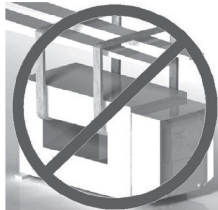
Incorrect Method of Lifting Detector
