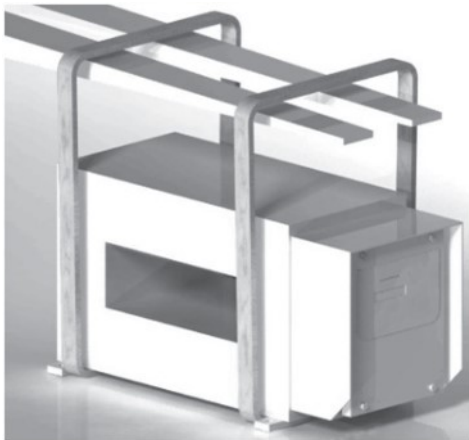
Correct Method of Lifting Detector
