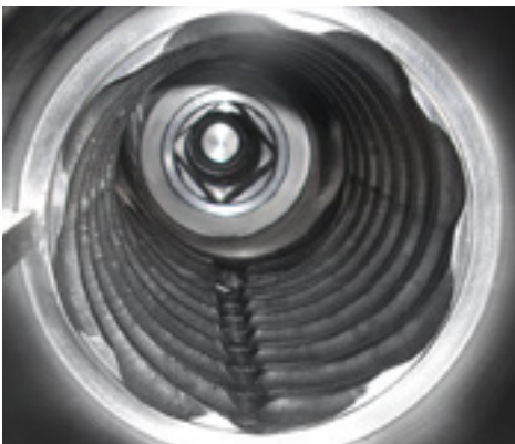
Solid, rust-free worm housing, robust drive bearing
